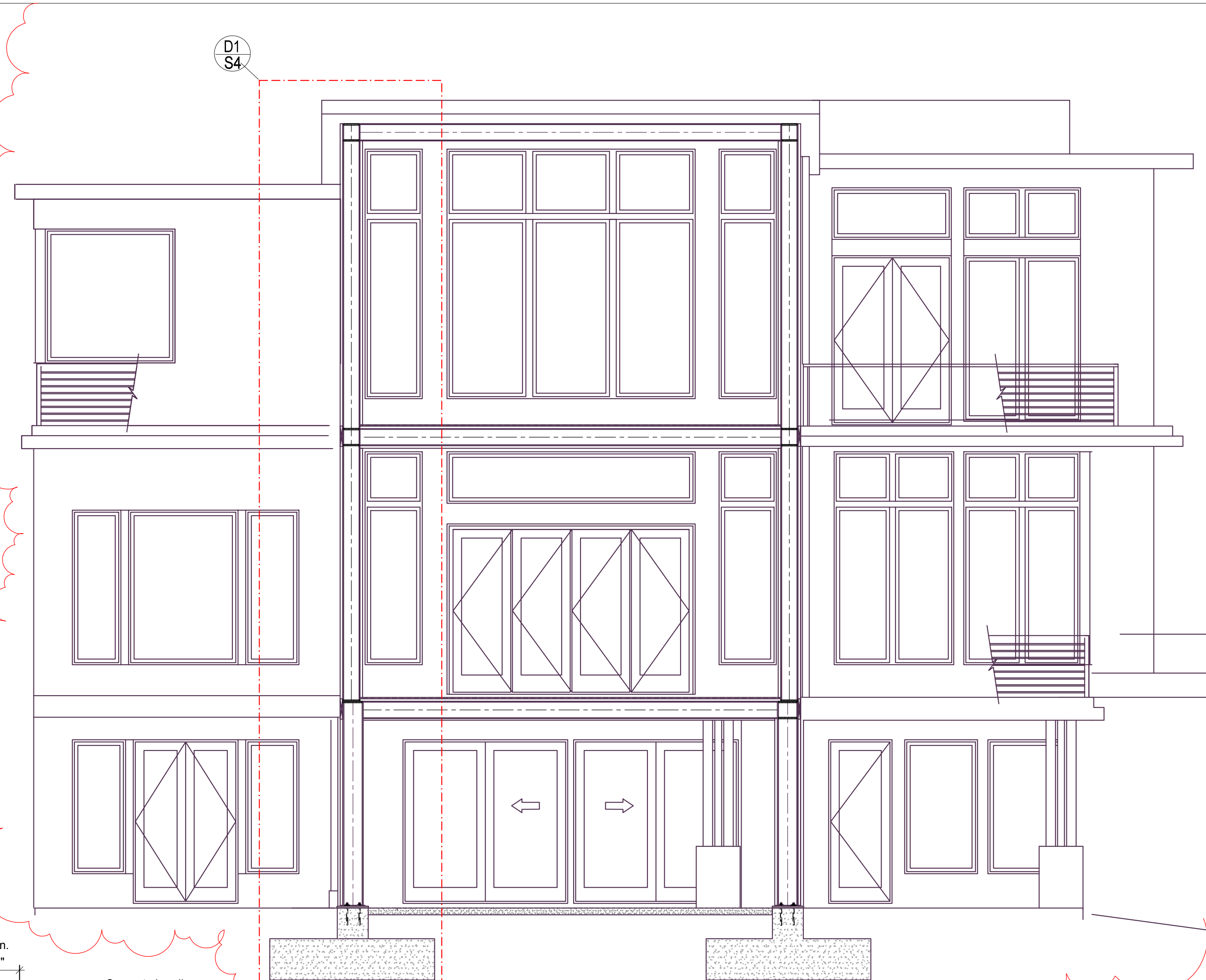
MOMENT FRAME ELEVATION M-M SCALE: 1/4" = 1'-0" (1:48)
